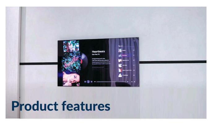
The **SBR 55LT-OLED** is a transparent screen Made of LG OLED screen, it supports the HD 1080 X 1920 output, it has a fine picture with high resolution, as well as a smooth video playback and built-in audio-video processing function producing a high-quality picture and sound quality output. The brightness of the display is 400cd/m², the light transmission is 40%, and the color range is wider. Industrial quality design, advanced technology, energy saving and environmental protection.
